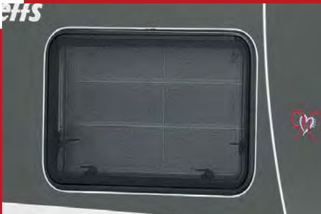
Sturdy, double-glazed flush-fitting windows with integrated blackout and mosquito blinds
