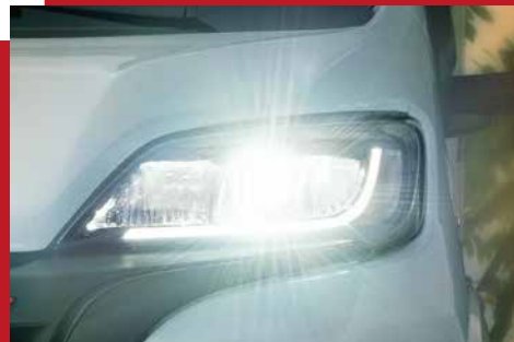
Full LED front headlights (daytime running lights, low beam, high beam and indicator lights)
