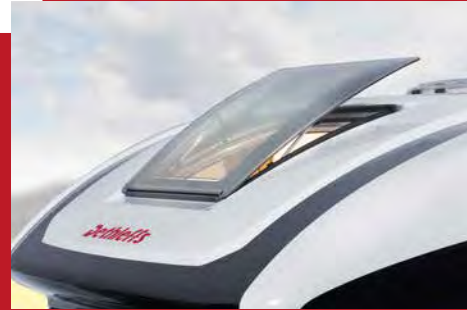
The openable window in the cab hood allows more light and air into the vehicle
