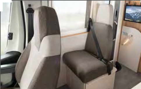
In DBL and EBL layouts, the transverse seating can be converted into a seat with safety belt
