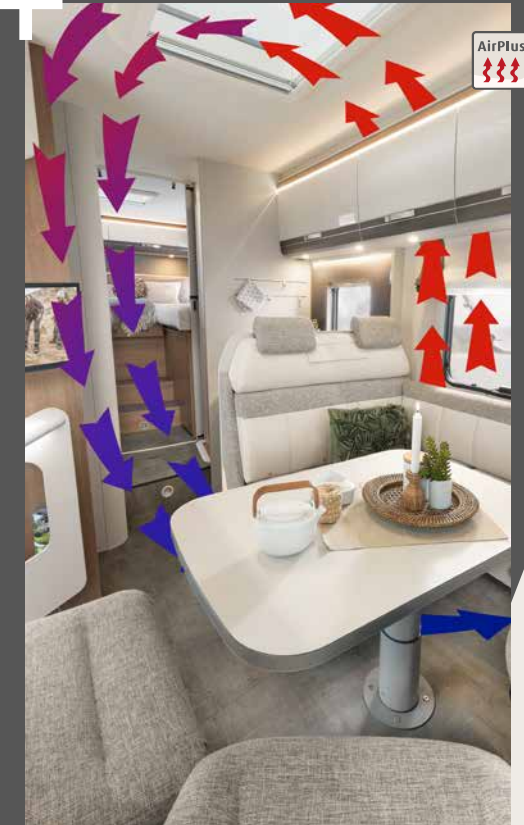
The AirPlus system avoids any condensation behind the lockers
